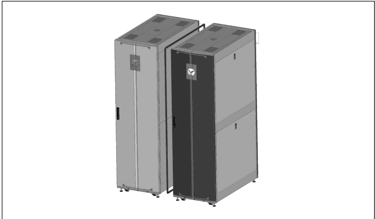
Figure 4.11 Baying gasket location
