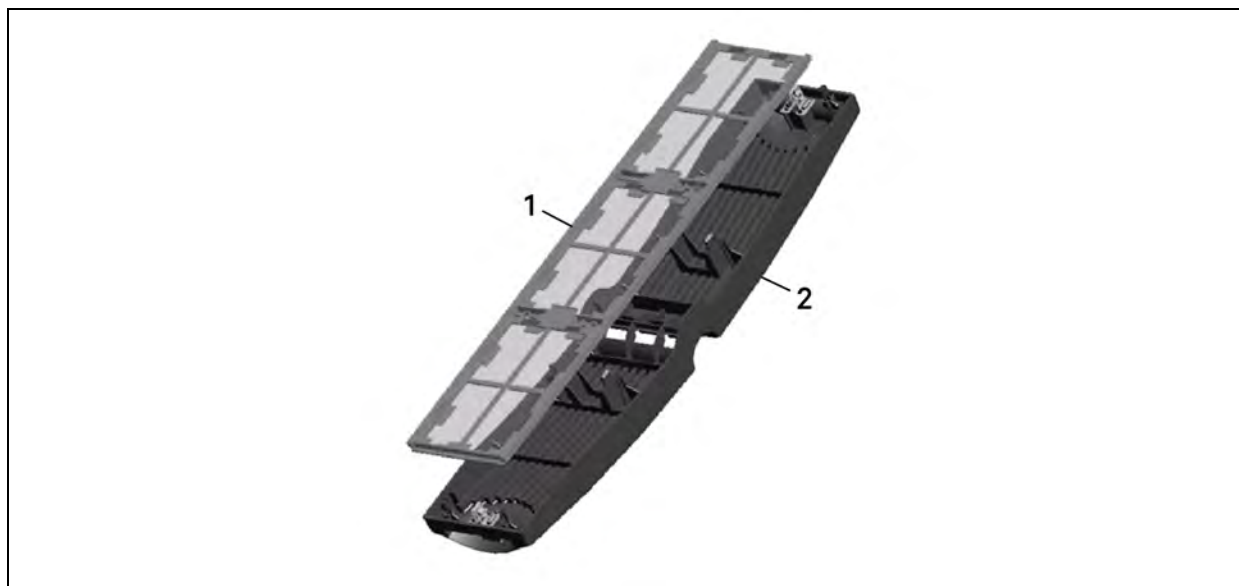
Figure 7.2 Replacing/Cleaning the bezel filter
