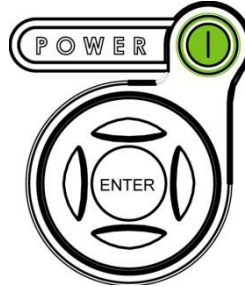
Figure 18 - CRT-400 Power and Arrow buttons
