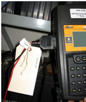
Figure 29 - Insert Resistance Test Leads Left Side CRT
