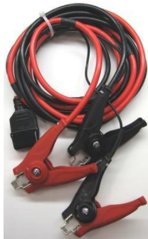
Figure 28 - Resistance Test Lead Assembly Clamps
