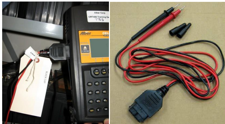
Figure 25 - Connect Voltage Test Leads
