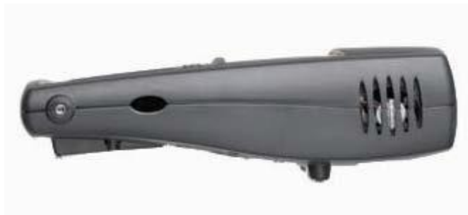
Figure 2 - Cellcorder Right Panel Connector/Infrared
