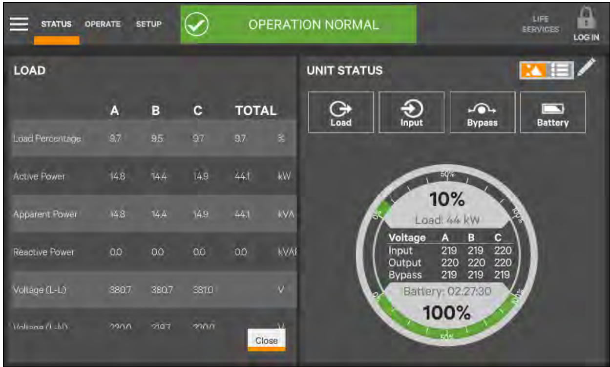
Figure 5.28 Unit Status-Load Details
