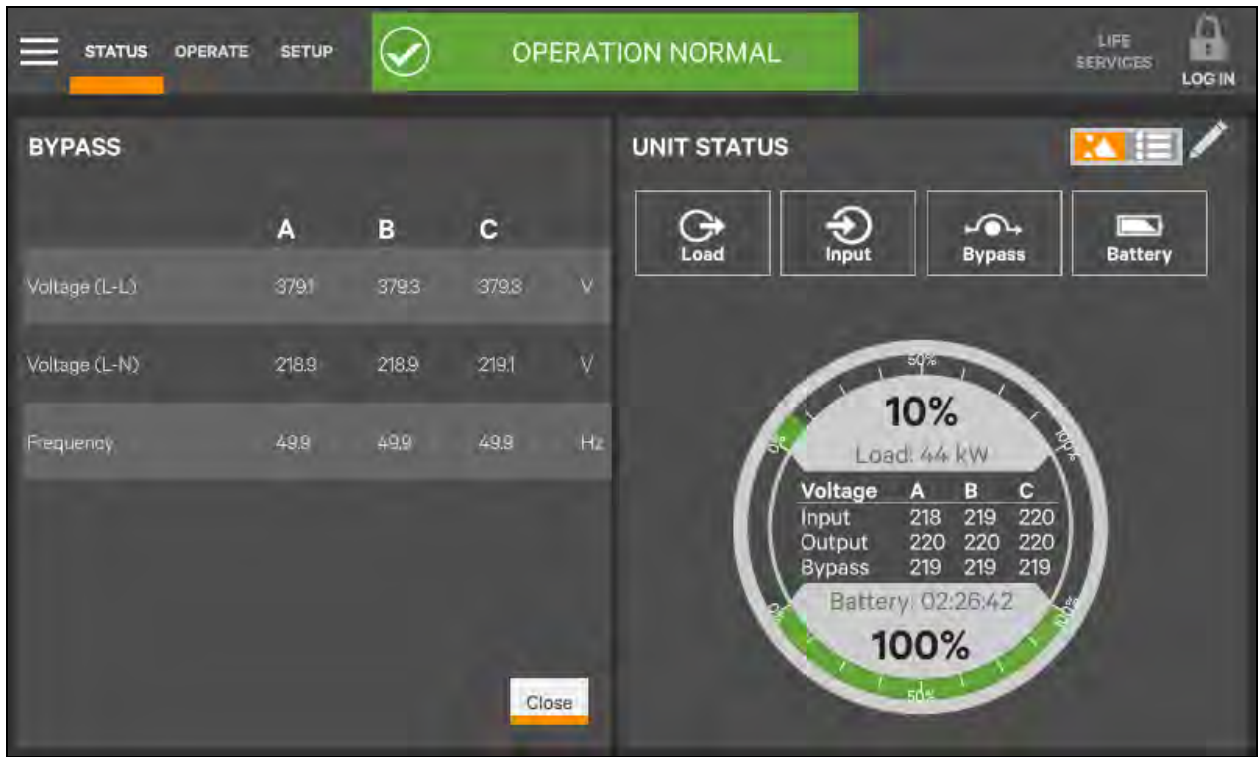
Figure 5.26 Unit Status-Bypass Details
