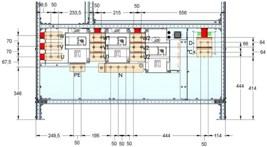
Figure 29 - Liebert EXL S1 500 kVA Customer power connections (front view)
