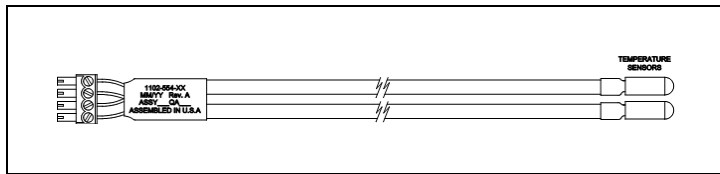
Figure 9.9 Ambient Temperature Connection on Rear of UXBM/50 Battery Module
