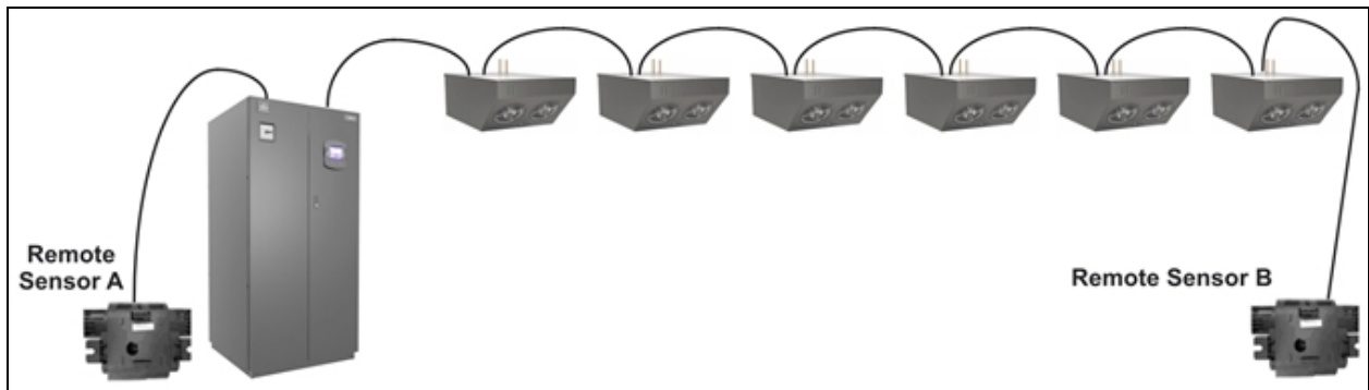
Figure 3.22 Liebert® XD System with CANbus
