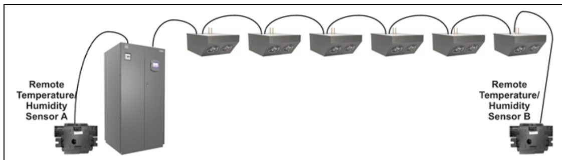
Figure 7.6 Liebert® XD System with CANbus
