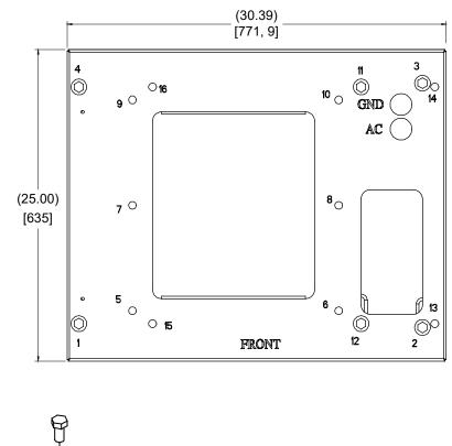
Figure 7.2 Pour-in-Place Pad Template Diagram F1009326 [inches (30Wx25D), mm (762Wx635D)]
