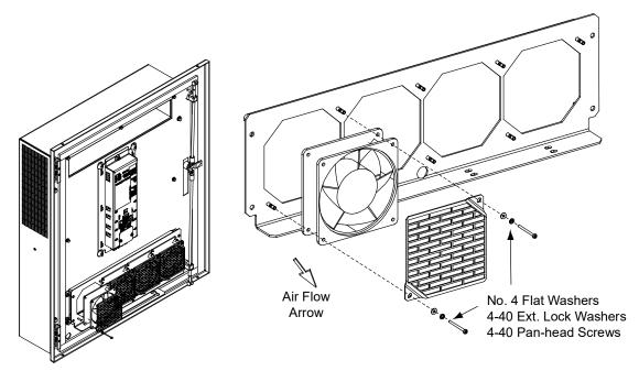
1450W Heat Exchanger Internal Fan Replacement
