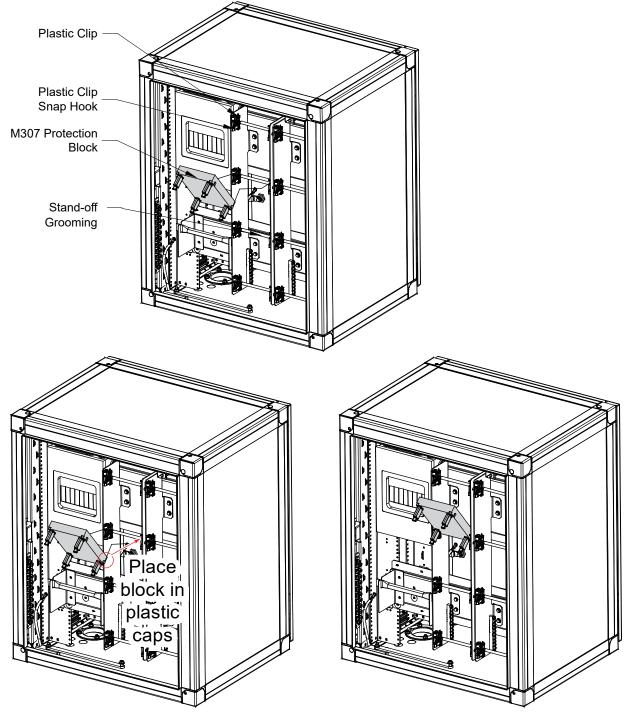
**Step 1:** Arrange the cables of the block over the stand-off grooming and place the M307 block on the plastic cap.
