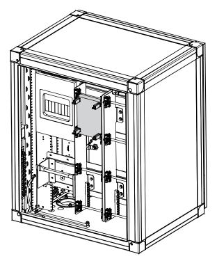
**Step 4:** Fix the M307 block by locking with snap hooks. To remove the block, move the snap hooks and pull out the block.
