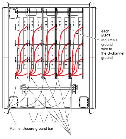
each U-channel has ground bar and ground wire
