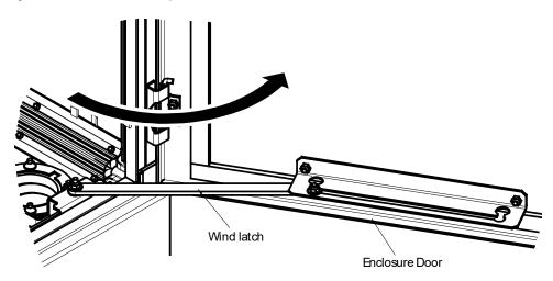
Figure 4.4 Releasing the Wind Latch Assembly
