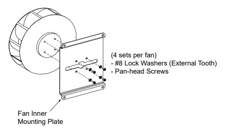
f) Attach the replacement fan to the fan inner mounting plate with the (4) sets of screws and star washers previously removed.
