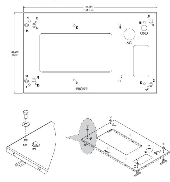
Figure 7.6 Pour-in-Place Pad Template Diagram - F1009331 [inches (42Wx25D), mm (1067Wx762D)]s
