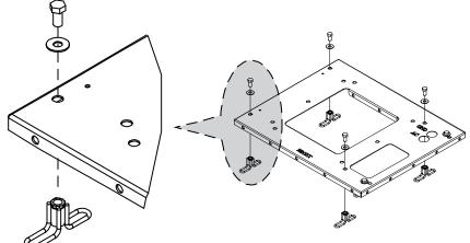
**NOTE!** See Figure 7.3 for the Reference Table on Drill Template (P/N 558205) and for locating correct mounting holes. Place hardware as shown in Figure 7.2 prior to placing pour-in-place pad template.
