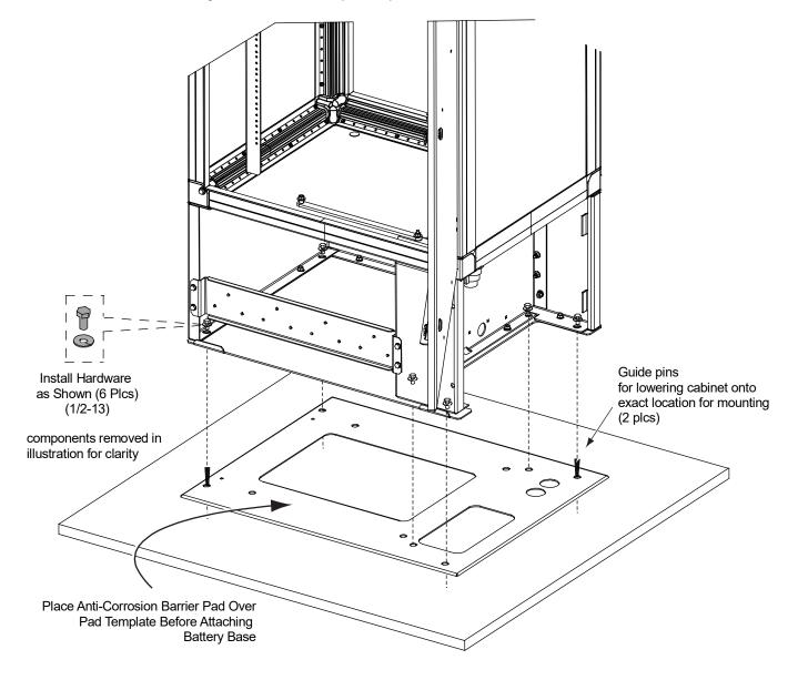
Figure 8.1 Attaching Enclosure to Pad - Enclosure with No Side Chamber (battery base shown, w/o battery base similar except (4) inner set of mtg. holes used - refer to pad template illustrations)
