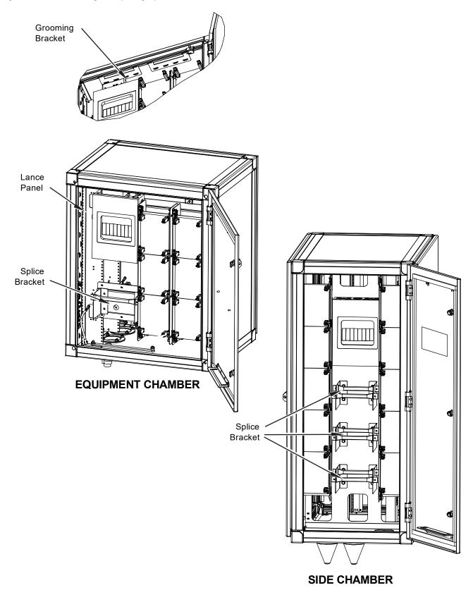
Figure 10.7 Cable Routing and Splicing Options for Protection Cables
