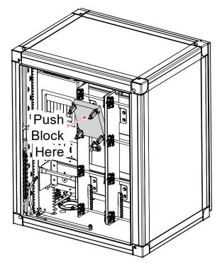
**Step 3:** Push the top surface of the M307 block towards the snap hooks.
