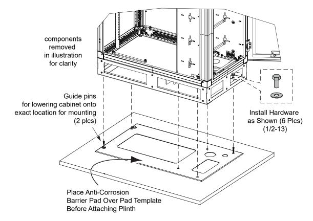
Figure 8.7 Attaching Enclosure to Pad - Enclosure with Two Side Chambers (with battery base shown, w/o battery base similar except (4) inner set of mtg. holes used - refer to pad template illustrations)
