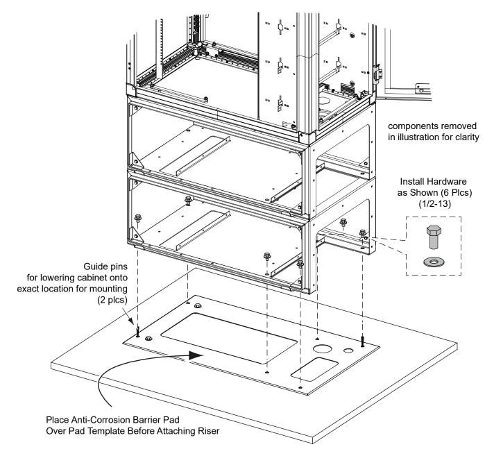
Figure 8.5 Attaching Enclosure to Pad - Enclosure with One Side Chamber (with riser installed - refer to pad template illustrations)
