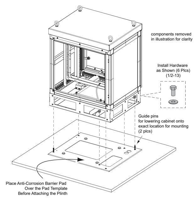
Figure 8.4 Attaching Enclosure to Pad - Enclosure with One Side Chamber (battery base shown, w/o battery base similar except (4) inner set of mtg. holes used - refer to pad template illustrations)
