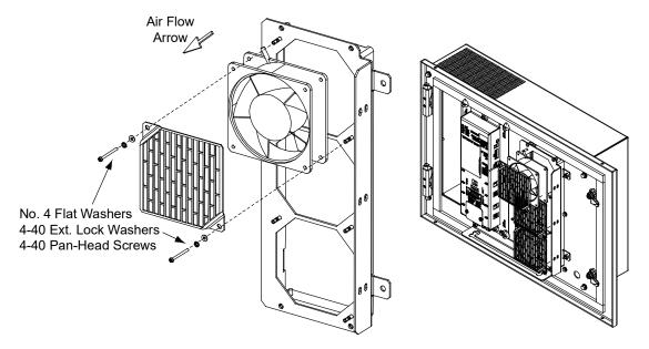
1000W Heat Exchanger Internal Fan Replacement
