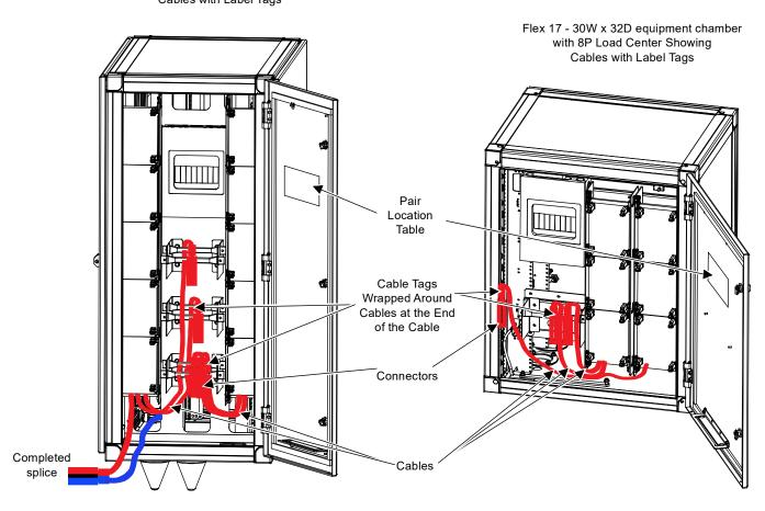
Flex 27 - 42W x 25D side chamber with 8P Load Center Showing Cables with Label Tags
