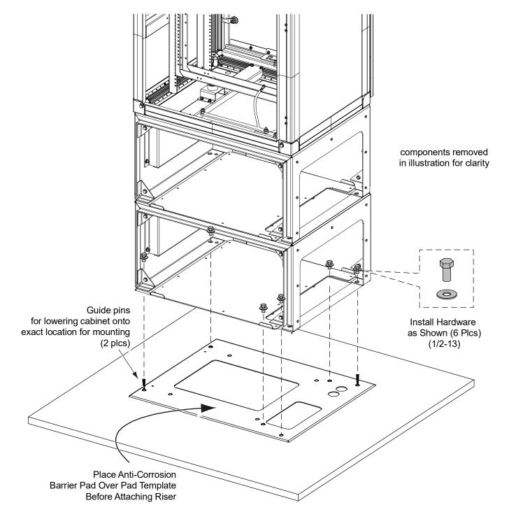
Figure 8.2 Attaching Enclosure to Pad - Enclosure with No Side Chamber (with riser installed - refer to pad template illustrations)
