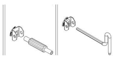
Figure 4.2 Swing Handle Latch with Provision for Padlock
