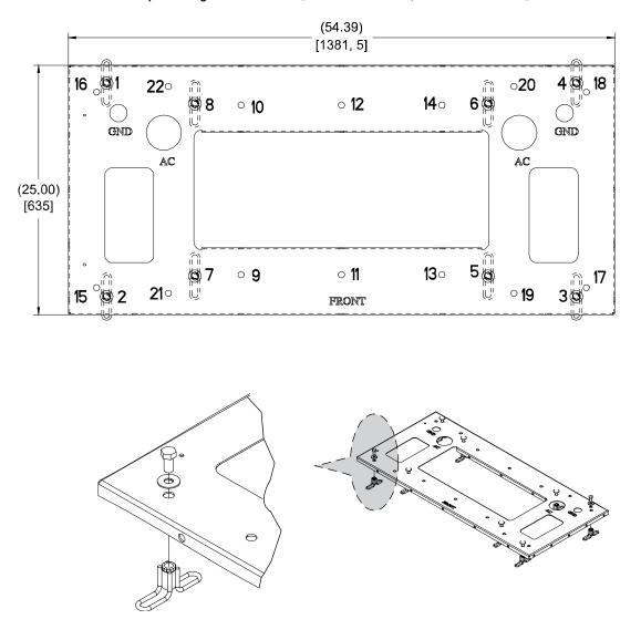
Figure 7.10 Pour-in-Place Pad Template Diagram - F1009333 [inches (54Wx25D), mm (1372Wx762D)]
