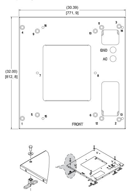
Figure 7.4 Pour-in-Place Pad Template Diagram F1009332 [inches (30Wx32D), mm (762Wx813D)]
