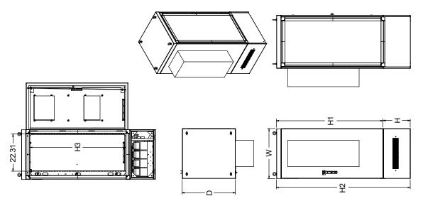
Figure 2.3 Enclosure Assembly with Battery Chamber (42"x32", 42"x25")
