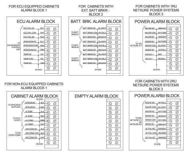
NOTE: ALARM BLOCKS ARE INSTALLED FROM TOP TO BOTTOM. TOP ALARM BLOCK IS POSITION 1 AND SHOULD BE ALARM BLOCK 1
