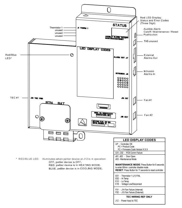
Figure 14.12 +24Vdc and -48Vdc ECU Controlling Two (2) TECs
