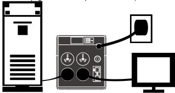
Plug the loads into the battery backup outlets on the rear of the UPS.
