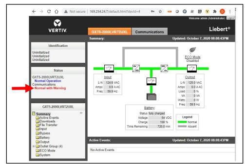
12. After logging in, the Status area on the left-hand side of the appliance screen may indicate a Normal with Warning Communications status.
