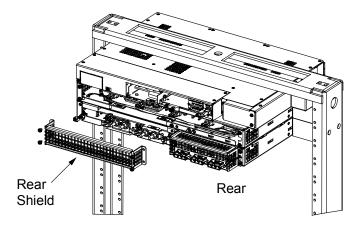
4. Remove rear shield from the expansion module mounting assembly.
