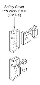
Figure 5: Replacing a Bullet Nose Circuit Breaker (List BA, NA)
