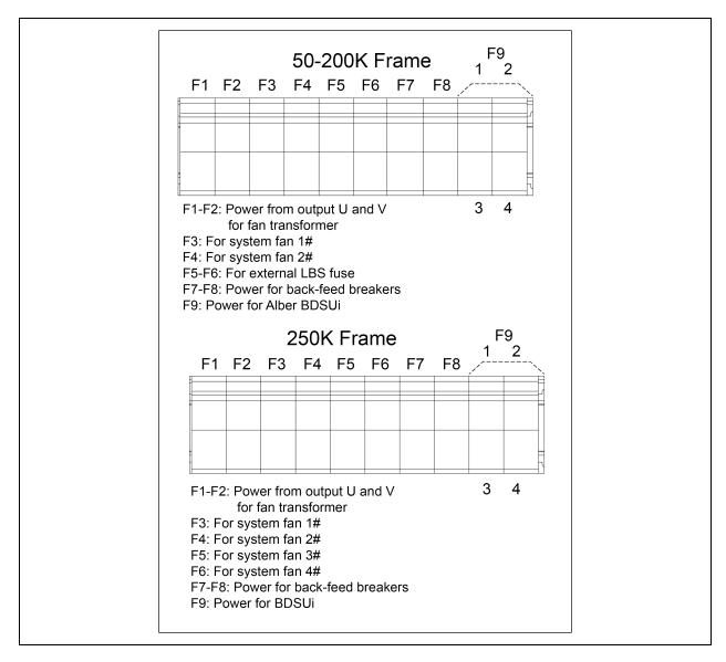
Two fuse blocks provide power for the back-feed breakers (standard) and the Vertiv<sup>TM</sup> Alber<sup>TM</sup> BDSUi (optional). The accessory fuse holders are shown in **Figure 5.2** on page 46 and **Figure 5.4** on page 48.
