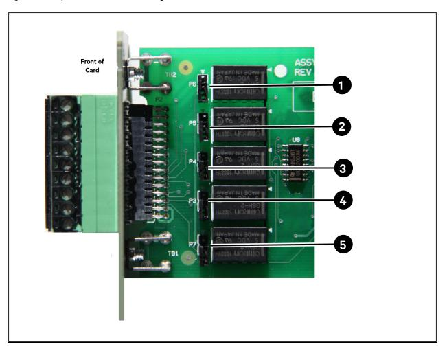
By default all five jumpers have shunts installed. The two pins are shunted together to provide the functions shown in **Table 6.3** below, allowing relay commons to be tied together.
