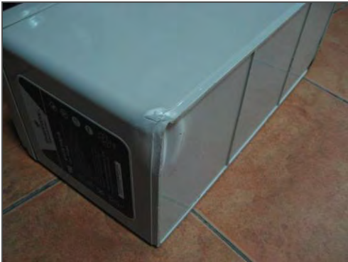
Battery damaged during handling or transportation
