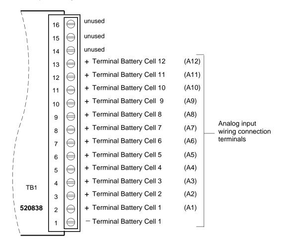
Analog input designations A1 through A12 as shown are for the circuit card only. The actual analog channel number depends upon the quantity of analog and temperature circuit cards installed and location of this analog circuit card in the system network.
