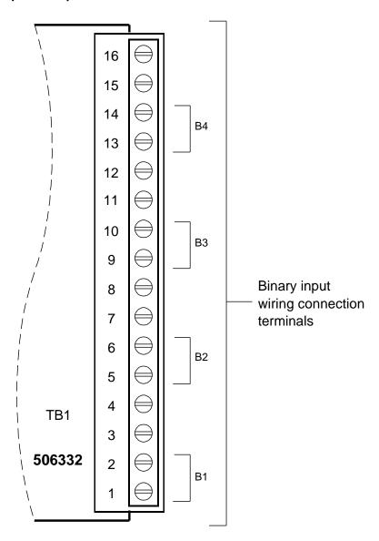
Binary input designations B1 through B4 as shown are for the circuit card only. The actual binary channel number depends upon the quantity of binary circuit cards installed and the location of this binary circuit card in the system network.
