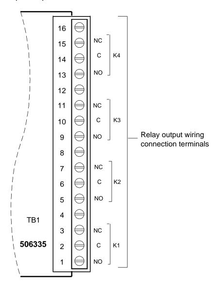
Relay designations K1 through K4 as shown are for the circuit card only. The actual relay channel number depends upon the number of relay circuit cards installed and the location of this relay circuit card in the system network.
