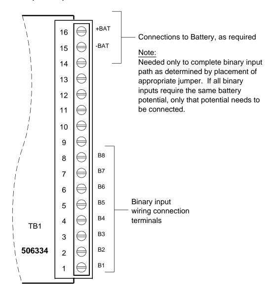
Binary input designations B1 through B8 as shown are for the circuit card only. The actual binary channel number depends upon the quantity of binary circuit cards installed and the location of this binary circuit card in the system network.
