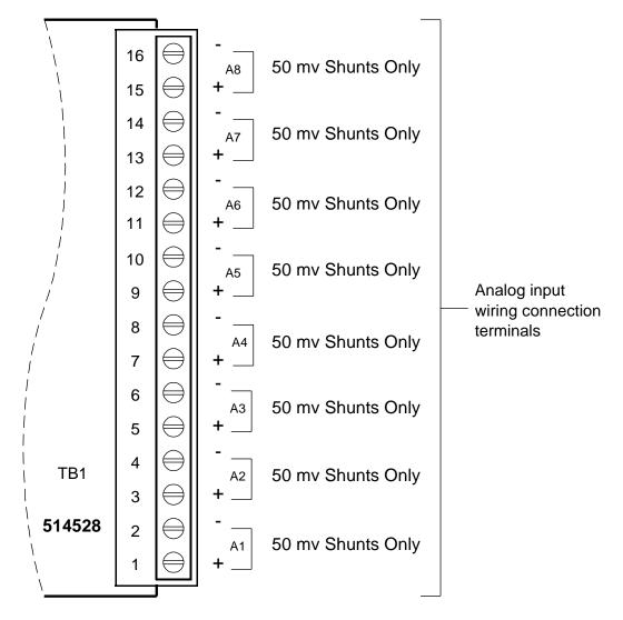
Analog input designations A1 through A8 as shown are for the circuit card only. The actual analog channel number depends upon the quantity of analog and temperature circuit cards installed and location of this analog circuit card in the system network.
