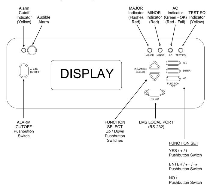
Navigating the MCA is an easy process. You just have to remember a few key combinations (as shown in the following chart). The symbols that appear at the end of the fourth line of the display indicate which keypad buttons can be pressed at any given time.
