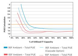
\*CRV inlet air temperature 75° F. PUE is a measure of how efficiently a computer data center uses its power; specifically, how much of the power is actually used by the computing equipment (in contrast to cooling and other overhead).
