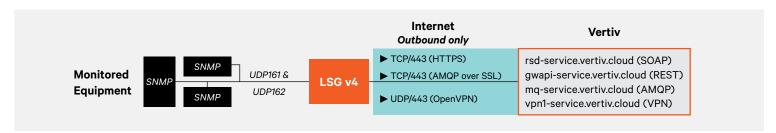
The gateway performs several critical functions from translating SNMP protocols to encrypting, processing, managing, and filtering data. It does this by optimizing system performance through the collected operational data gathered and processed in real-time. SNMP is primary protocol supported for remotely monitoring devices. The collected data is normalized and then sent to the Vertiv cloud securely over the internet via AMQP over SSL.
