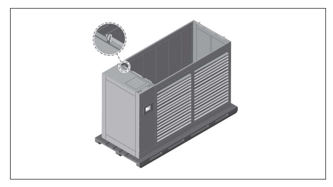
Figure 4.4 Rigging-fastener Eye Nut Installed
