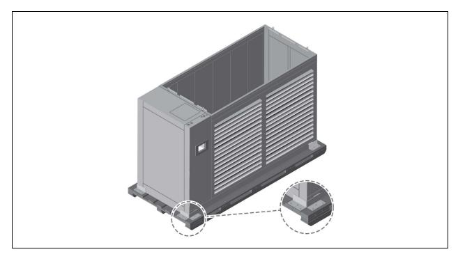
2. Using the provided rigging-fastener kit and the instructions included in the kit, install the rigging hardware for lifting the unit from the skid. **Figure 4.4** below, shows an example of one of the eye nuts installed.
