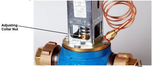
**Manual Flushing**—The valve may be flushed by rotating the socket head screw clockwise. This screw must be in the OUT position (counterclockwise) for normal valve operation.
