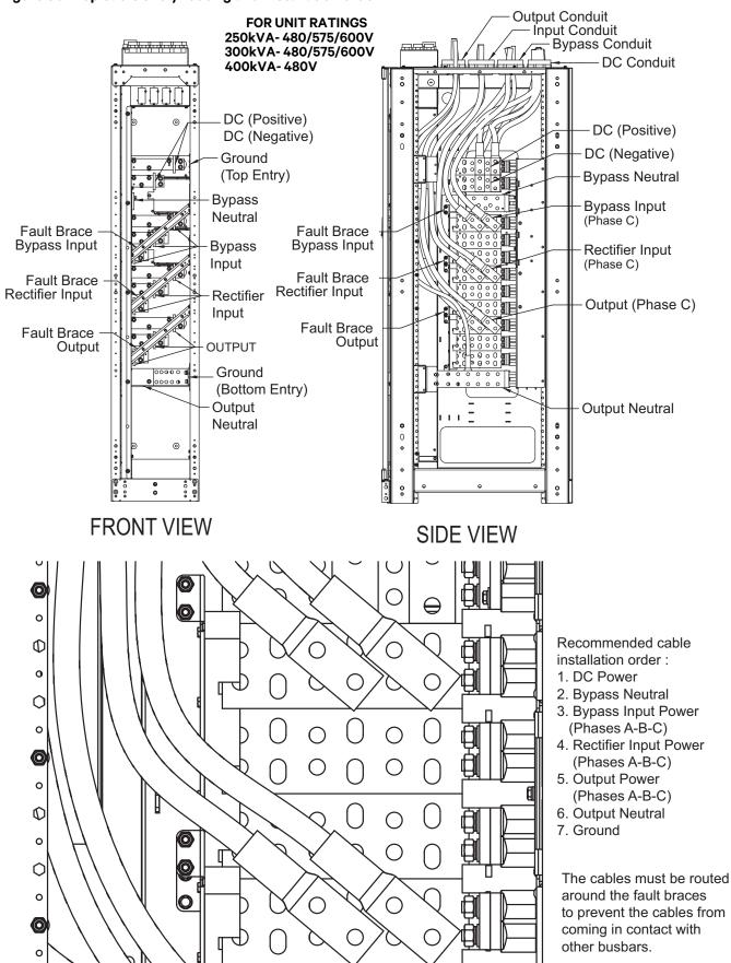
Figure 31 Bottom cable entry routing and installation order
