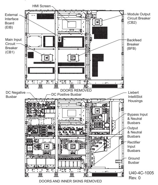
Figure 25 Main components, 400kVA, 575V/600V Liebert NXL with DC I/O cabinet
