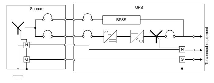
Figure 10 Grounding diagram, three-wire multi-module system
