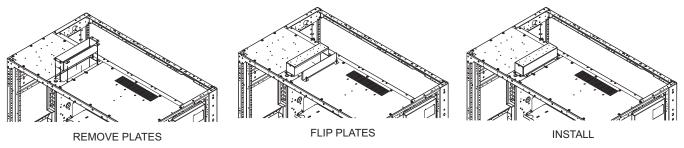
Low-voltage cables can be installed through the top of each unit. The entry conduit landing plate is shipped inverted. To install, remove conduit plate, flip and reinstall. Removal of side plate is for access to pull wires.
