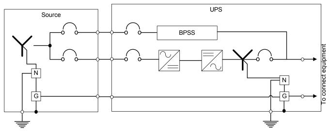
Figure 9 Grounding diagram, four-wire single-module system
