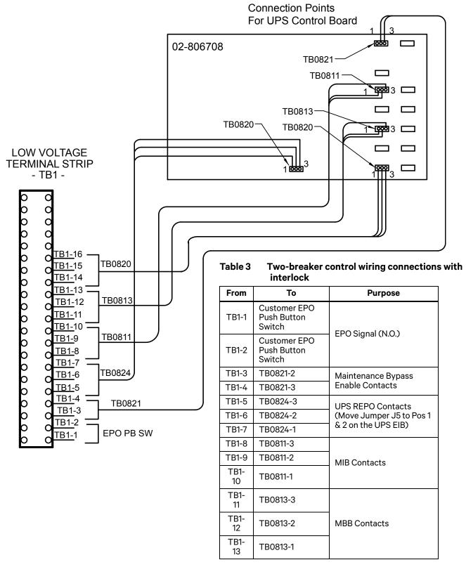
Figure 13 Liebert NXL two-breaker Maintenance Bypass Cabinet control wire diagram with interlock
