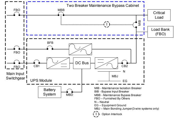
Figure 3 Liebert NXL two-breaker Maintenance Bypass Cabinet, three-input, attached
