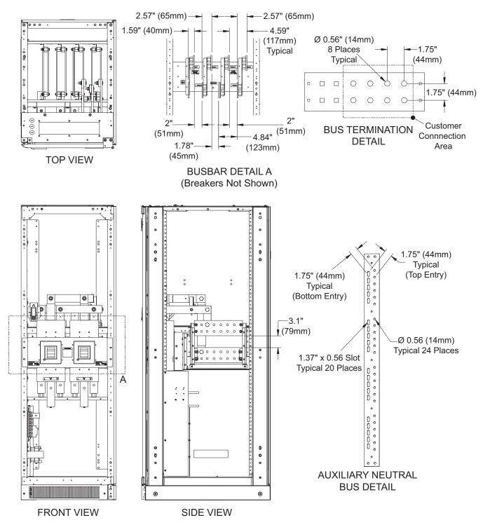
Figure 9 Liebert NXL two-breaker Maintenance Bypass Cabinet—400kVA and 500kVA terminal details
