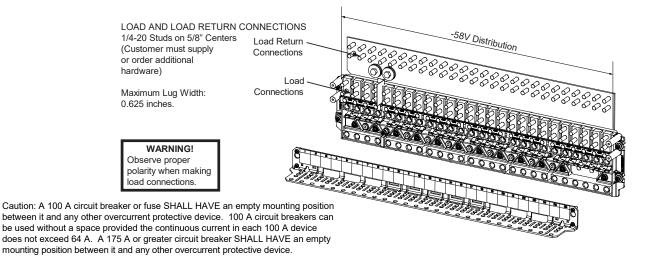
Figure 5.12 List FG: -48 VDC / -58 VDC Distribution Panel, (14) -48 VDC Bullet/TPS/TLS Circuit Breaker/Fuse Positions (with Return Busbar) and (12) -58 VDC Bullet/TPS/TLS Circuit Breaker/Fuse Positions (with Return Busbar)
