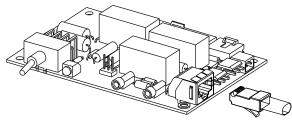
CAN termination plug P/N 548398 must be installed if an external device is not connected to the system.
