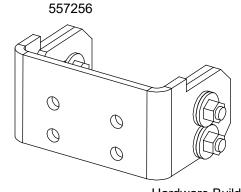
Hardware Build Up 3/8-16 x 1-1/2" Bolt 3/8" Flat Washer **Busbar Link Spacer Busbar Link** 3/8" Flat Washer 3/8" Belleville Lock Washer 3/8-16 Nut
