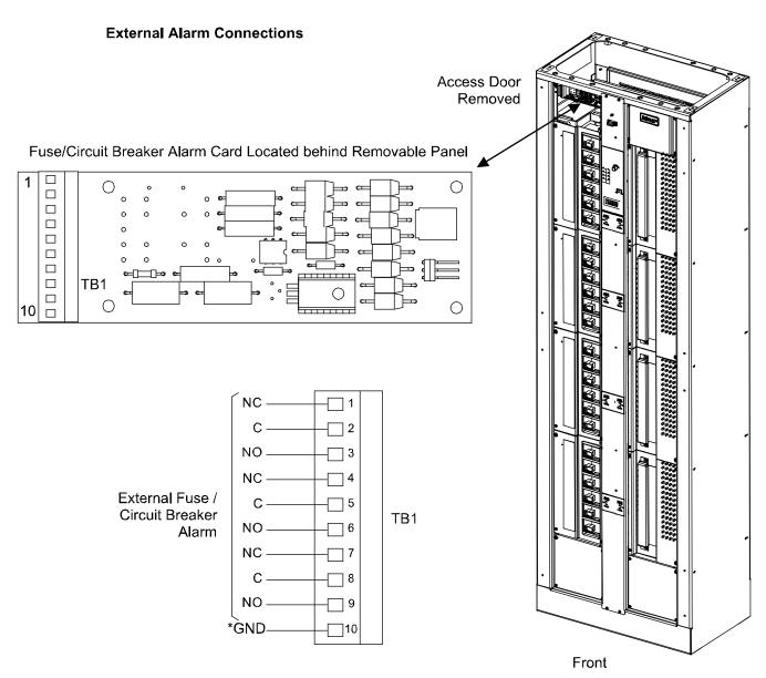
\* May be strapped to terminal 2, 5, or 8 to provide switched ground, if required.
