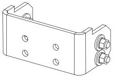
Hardware Build Up 3/8-16 x 1-1/4" Bolt 3/8" Flat Washer Busbar Link 3/8" Flat Washer 3/8" Lock Washer 3/8-16 Nut
