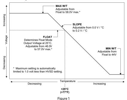
Typical Float Charge Thermal Characteristics
