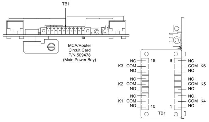
MCA Customer Alarm Relay Circuit Card P/N 514348 (Main and/or Supplemental Power Bays)
