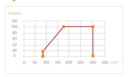
Figure 1: Output Power vs. Input Voltage and Vo > 48 V at Temp <45°C
