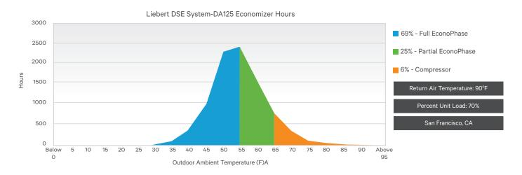
The prescriptive requirement for Computer Rooms is further defined in Section 140.9, where either integrated air economizers or integrated water economizers are capable of providing 100 percent of the expected system cooling load. For water economizers, this must be met with outside air temperatures of 40°F dry-bulb/35°F wet-bulb conditions and below.
