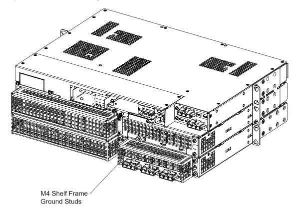
Figure 5.2 System Shelves Frame Grounding Connection Points
