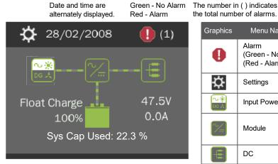
the total number of alarms. Graphics Menu Name Description Alarm View active alarms and (Green - No Alarm) alarm history. (Red - Alarm) Gain access to the NCU Settings Controller's settings menus. View AC. Solar. DG. and Input Power Wind related information. View rectifier, solar converter, Module and converter module related information. View DC equipments DC related information. View battery related Battery information.
