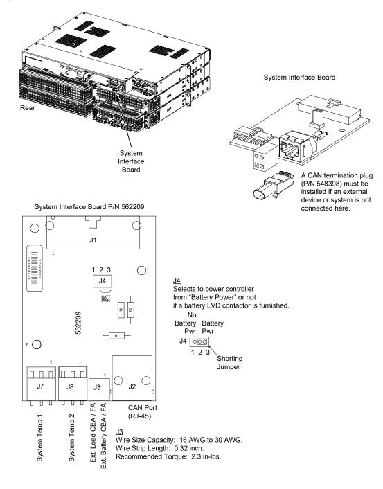
Figure 5.6 System Interface Circuit Card Connections
