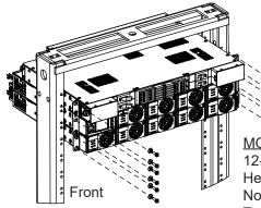
MOUNTING HARDWARE 12-24 x 3/4" Thread Forming Hex Head Screw No. 10/12 Ground Washer Torque: 65 in-lbs.
