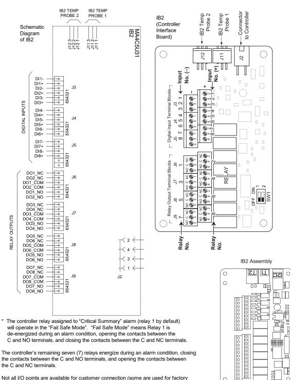
Not all I/O points are available for customer connection (some are used for factory system connections).
