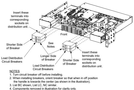
Figure 3.19 Installing Bullet-Nose-Type Battery Disconnect and Load Distribution Circuit Breakers (List BA, NA)
