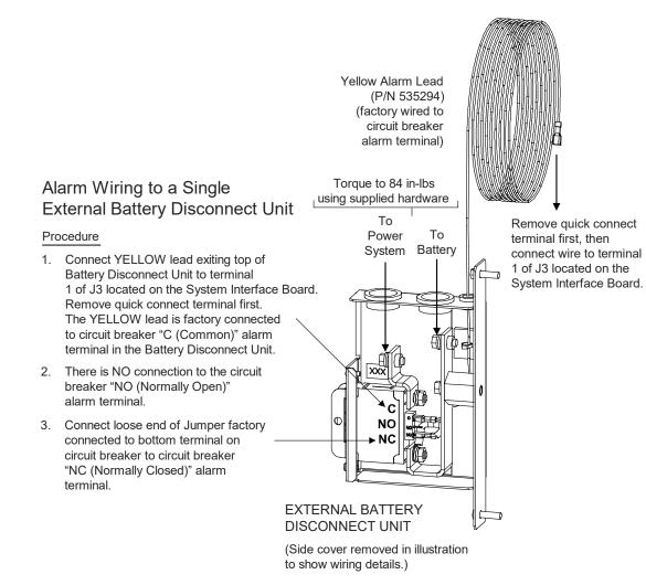
Figure 24 Circuit Breaker Alarm Connections to External Battery Disconnect Unit (cont'd from previous page)
