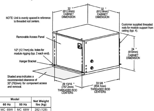
Figure 14 Cabinet and floor planning dimensional data—Split system—5-ton water/glycol-cooled condensing unit
