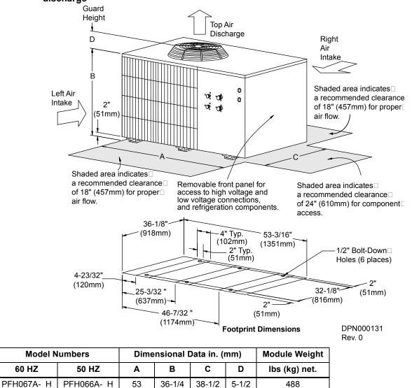
Figure 16 Cabinet and floor planning dimensional data—Propeller fan condensing modules—Vertical air discharge
