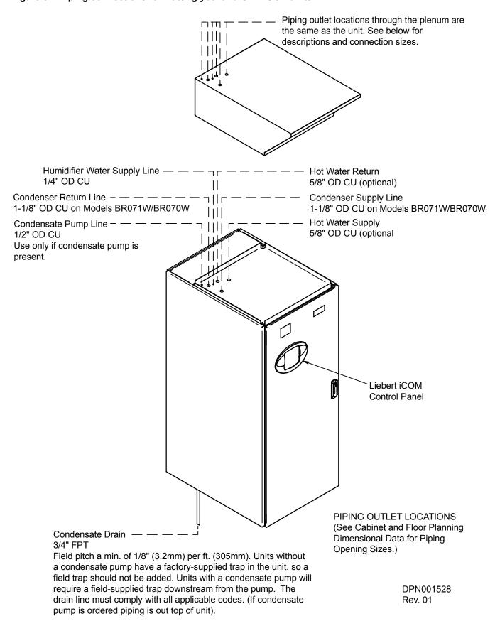
Figure 7 Piping connections for chilled water self-contained units
