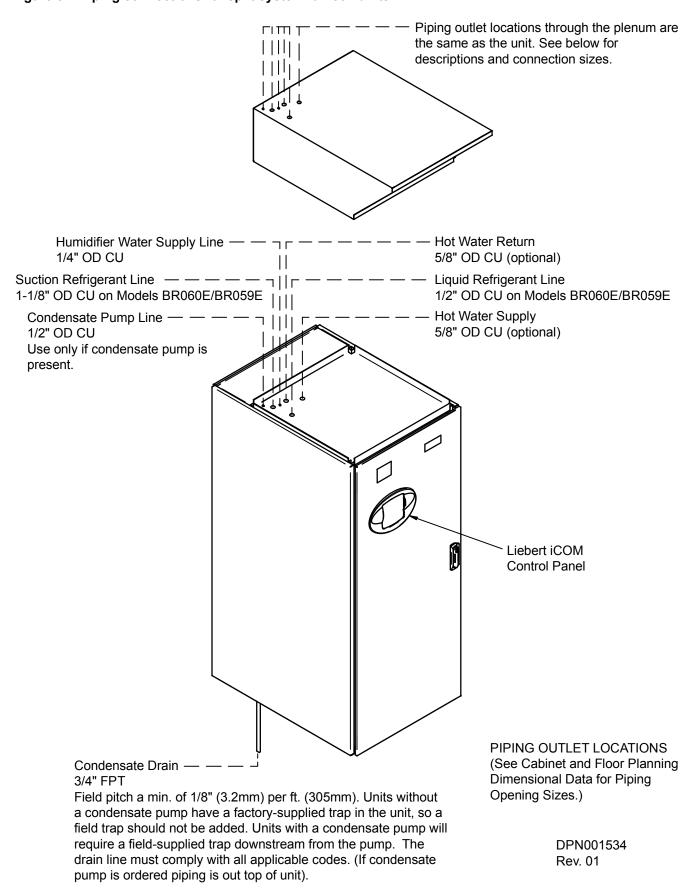
Figure 6 Piping connections for water/glycol and GLYCOOL units
