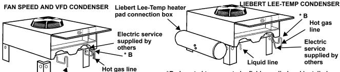
Secure each leg to condenser frame at all points shown using hardware provided.
