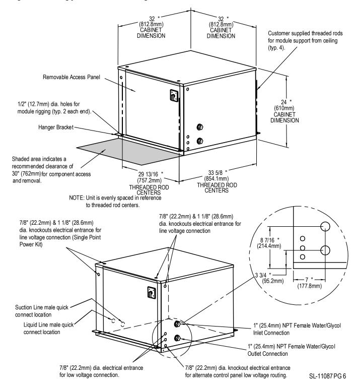
Figure 34 Water/glycol-cooled condensing unit (con't.)
