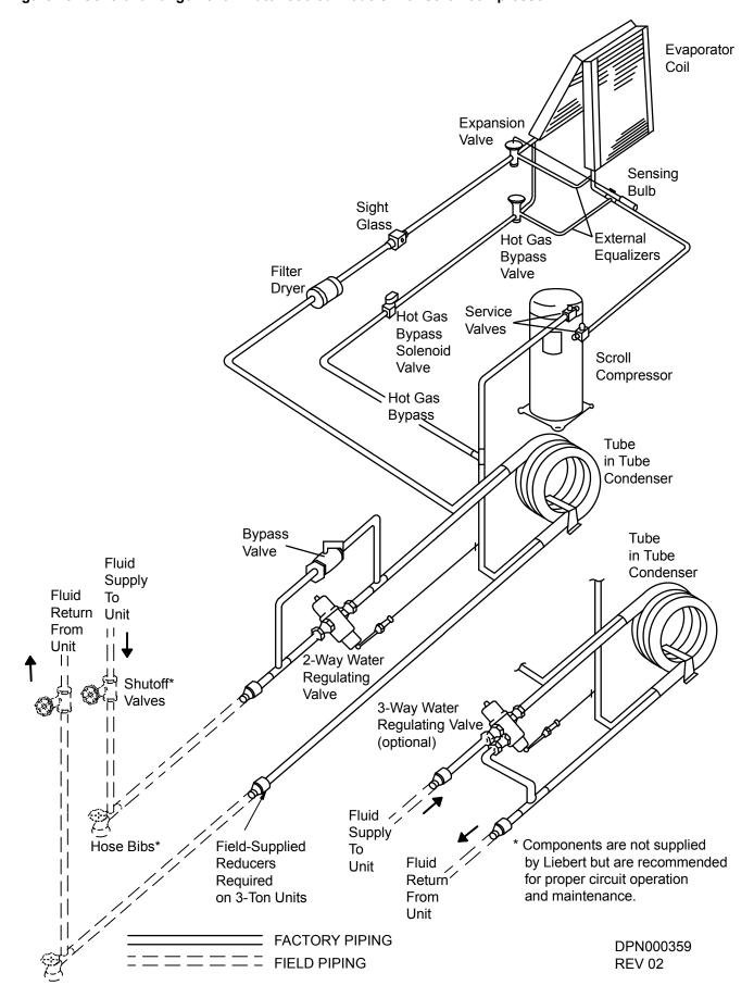
Figure 16 General arrangement diagram—Water-cooled models with digital scroll
