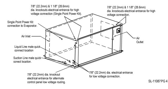
Figure 31 Centrifugal air-cooled condensing unit dimensional data (con't.)
