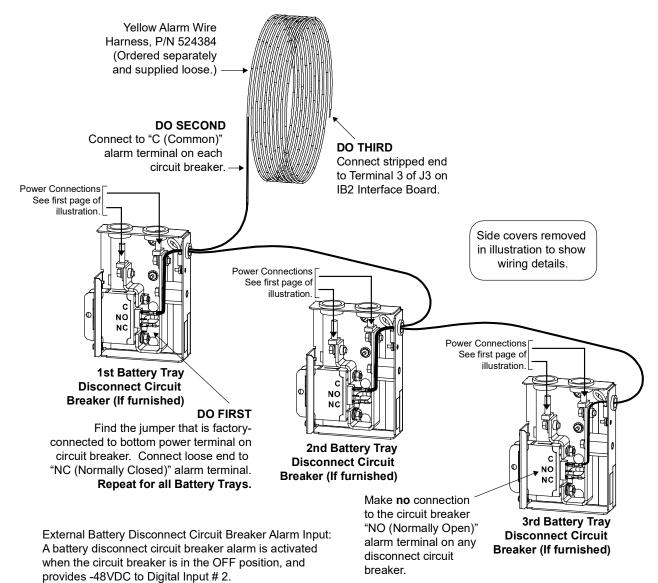
**BREAKER ALARM CONNECTION** Alarm Cable Shelf List CONNECT YELLOW WIRE TO: on shelf Must order Cable 545495 NO 1 or 2 545495 YES R-BK Lead of 545495. Splice and heat shrink tubing included with 545495 Pin 3 of J3 on customer interface BD (negative side of Digital Input # 2) NO 541311 5 or 6 O-R Lead of 541311. Splice and heat shrink tubing included with 541311 YES
