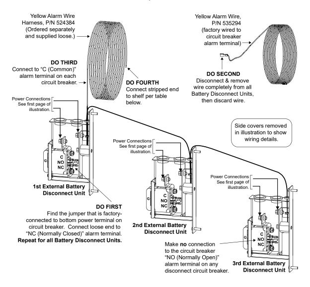
External Battery Disconnect Circuit Breaker Alarm Input: A battery disconnect circuit breaker alarm is activated when the circuit breaker is in the OFF position and provides -48VDC to Digital Input #2.
