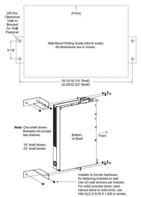
Figure 3.6 Vertical Wall Mounting, List 5 or 6
