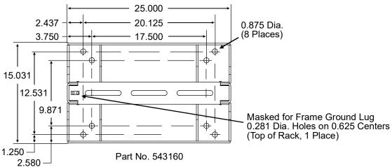
Figure 3.2 Relay Rack Floor Mounting Dimensions - 19" (dimensions are in inches)
