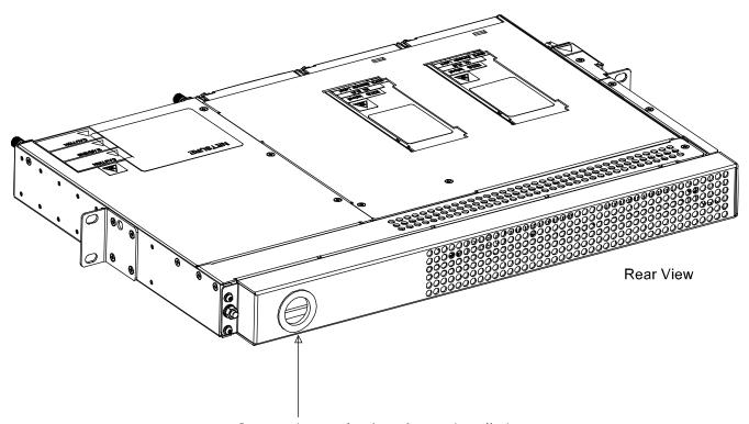
Connect battery leads to factory installed leads exiting the shelf here. These leads are factory terminated in an Anderson connector. A mating half to this connector is provided for connection to customer battery leads. External battery cables are also available to connect 1 (List 71 or 73) or 2 (List 72) strings of batteries to the system.
