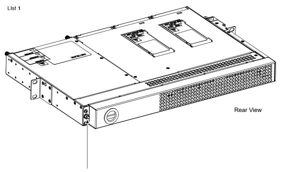
Connect a frame grounding lead to this stud, if required.
