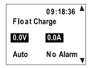
4. When initialization is complete, the Main screen displays voltage and current normally, and no alarms are active.
