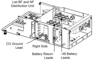
OBSERVE PROPER POLARITY WHEN MAKING BATTERY CONNECTIONS
