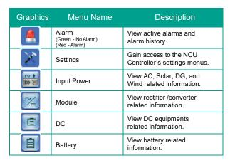
Press the UP and DOWN keys to highlight the desired Menu graphic in the Main Menu.
