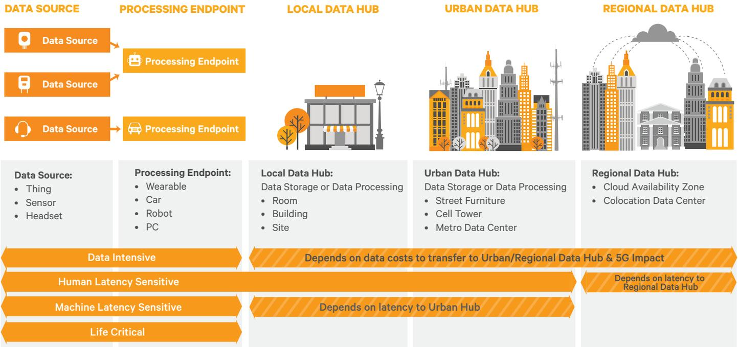
The metro hub leverages the existing telco infrastructure to support the local hub with longer-term data storage and more robust processing capabilities. The regional hub is likely to be a cloud data center operating in the same region as the local hub.
