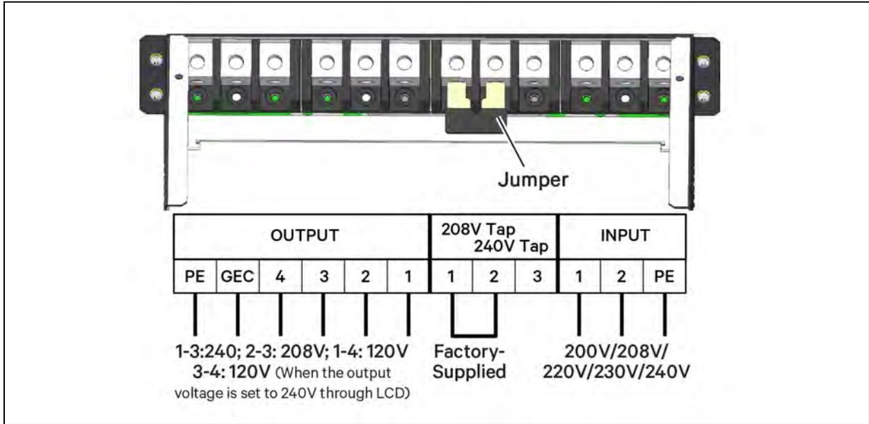
Refer to [Input cable selection for transformer-based frames \(50 Hz\)](#) on page 35 for configuring the output cable. For standard voltages, make the connections shown in [Key to Connection method on the previous page UPS output wiring](#) on the facing page.
