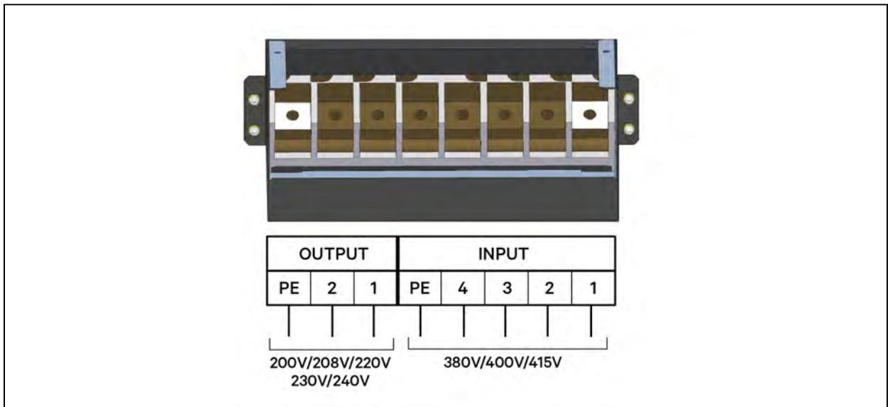
**Table 3.4 Key to Connection in single-phase input on the previous page and Connection in 3-phase input on the previous page UPS wiring**
