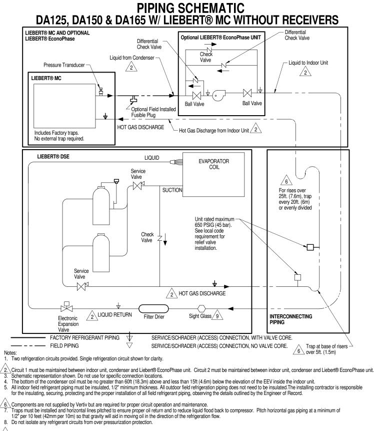
/9. Typical location for Sight Glass on DA150 and DA165. On DA125, Sight Glass is located between Filter Drier and Electronic Expansion Valve.
