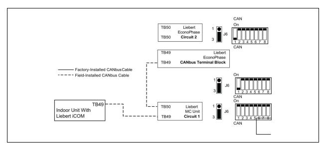
Figure 7.1 CANbus Cable Connections for Single Circuit System, PR050 and DA050
