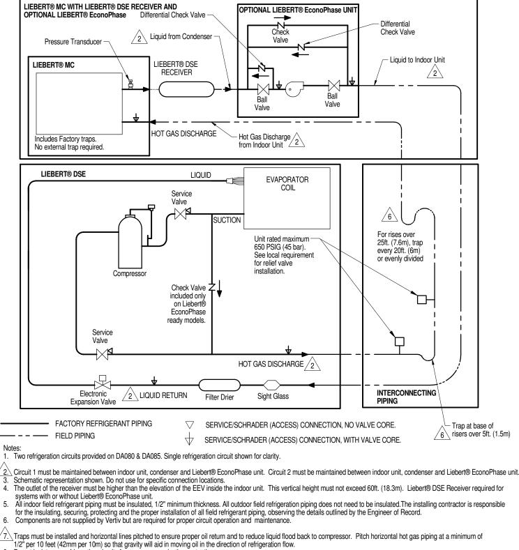
8. Do not isolate any refrigeration circuits from over pressurization protection.
